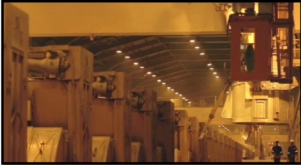
Figure 6. Metal tapping with PTA
