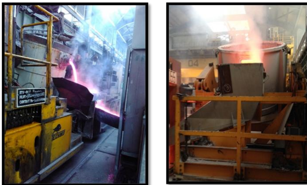
Figure 5. New practice of pouring metal from tapping vehicle instead of using crane.
